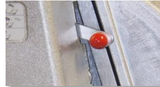
Manual activation lever of the fall arrest device
